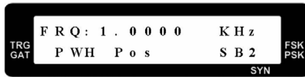
Square Wave Pulse Width Adjustment On and Output Positive Pulse
