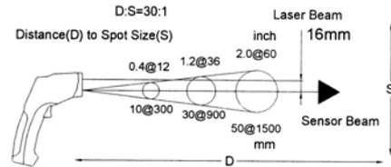
D = Distance (avoid exposure-laser radiation is emitted from this aperture) 30 : 1
